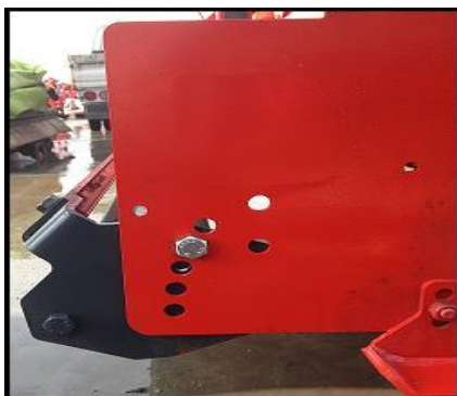
Figure 17 (6 stage shredder height adjustment holes)
